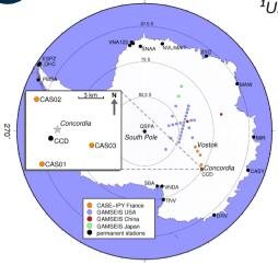
The CASE-IPY experiment is the French contribution to the IPY initiative POLENET (see map for locations of POLENET seismic stations). Its objective is the deployment of an array of seismometers between Concordia and Vostok, in Antarctica. Three prototype stations were deployed near Concordia in Jan 2008, and four profile stations in Jan 2010 (see photos below).
