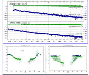
State-of-health of CASE stations. Data from the prototype stations, including state-of-health, is telemetered daily to Concordia. Plots show acquisition system voltage and temperature readings for 2010 and 2009. The stations are powered by solar panels and batteries. We have enough batteries to carry on recording approximately 1 month after the last sun-down
