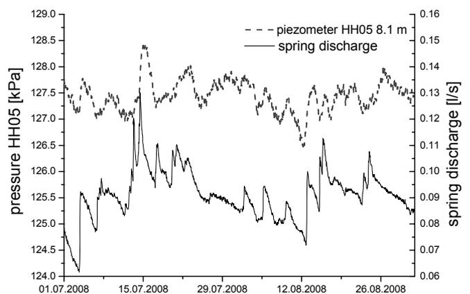
Figure 5. Concordance of pressure signal in HH05 and spring discharge is less than for piezometers of KB03, probably because both are located on the same topographic height.
