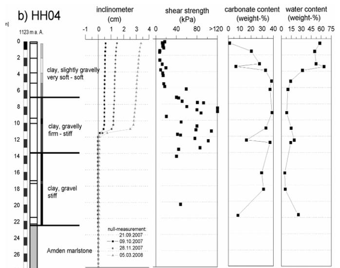
Figure 3. Simplified borehole log of HH04 with three major layers and results of field and laboratory investigations. A clear shear zone is detected in 11-12 m depth.
