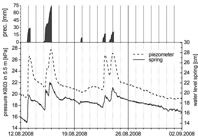
Figure 4. Relation of cumulative precipitation of single events, spring discharge (1127 m) and pressure changes about 300 m downhill in KB03 (1075 m) (see also Figure 1).
