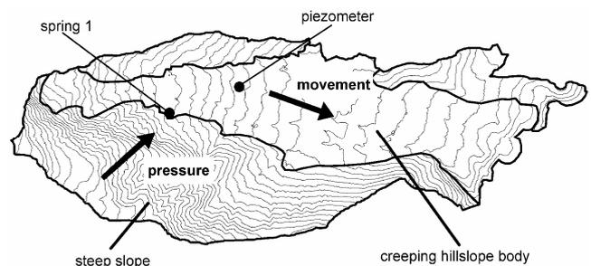
Figure 1. Pressure propagation from adjacent hydrological active hillslopes towards the creep mass which moves towards the east on the Heumös Slope.
