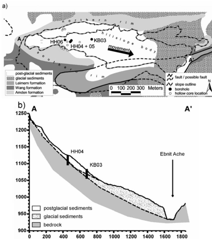
Figure 2. a) Geological map of the mass movement and adjacent hydrological relevant areas (northern and southern rim), arrow indicates direction of movement. b) Cross section in east-west direction and location of boreholes, the river Ebnit flows at the tow of the Heumös Slope.
