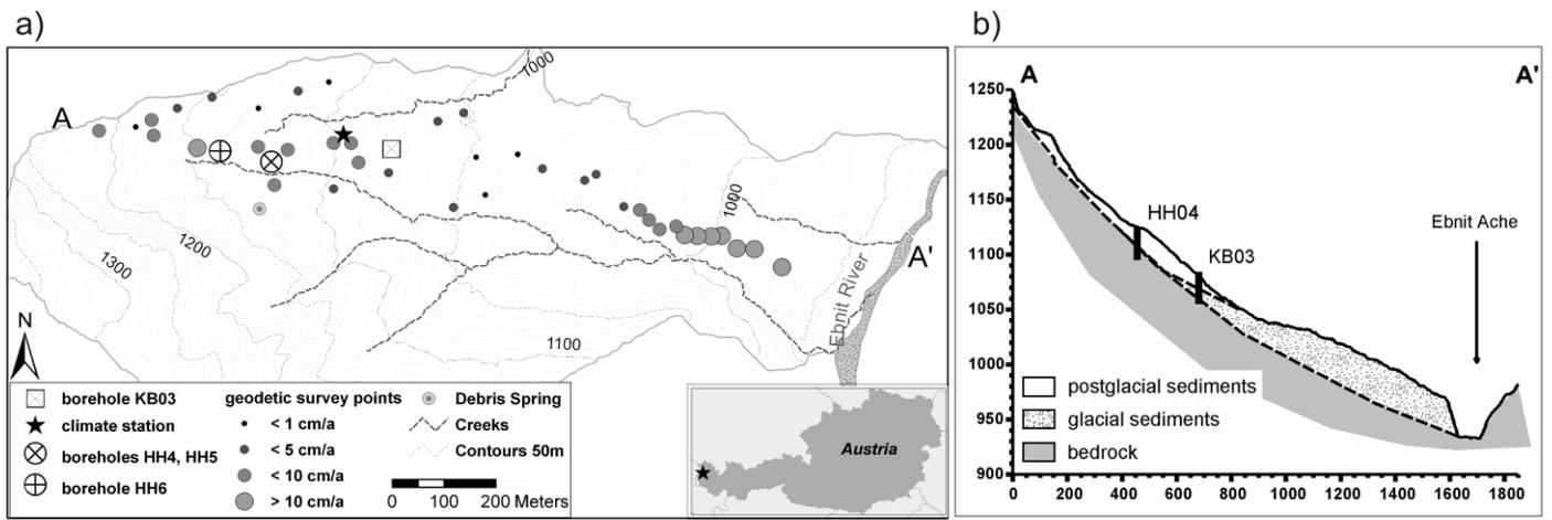
Figure 1. a) Map of the study area *Heumöser Hang* with locations of measurement network. The inset shows the location of the area in Austria. b) Schematic geological cross-section (W-E).
