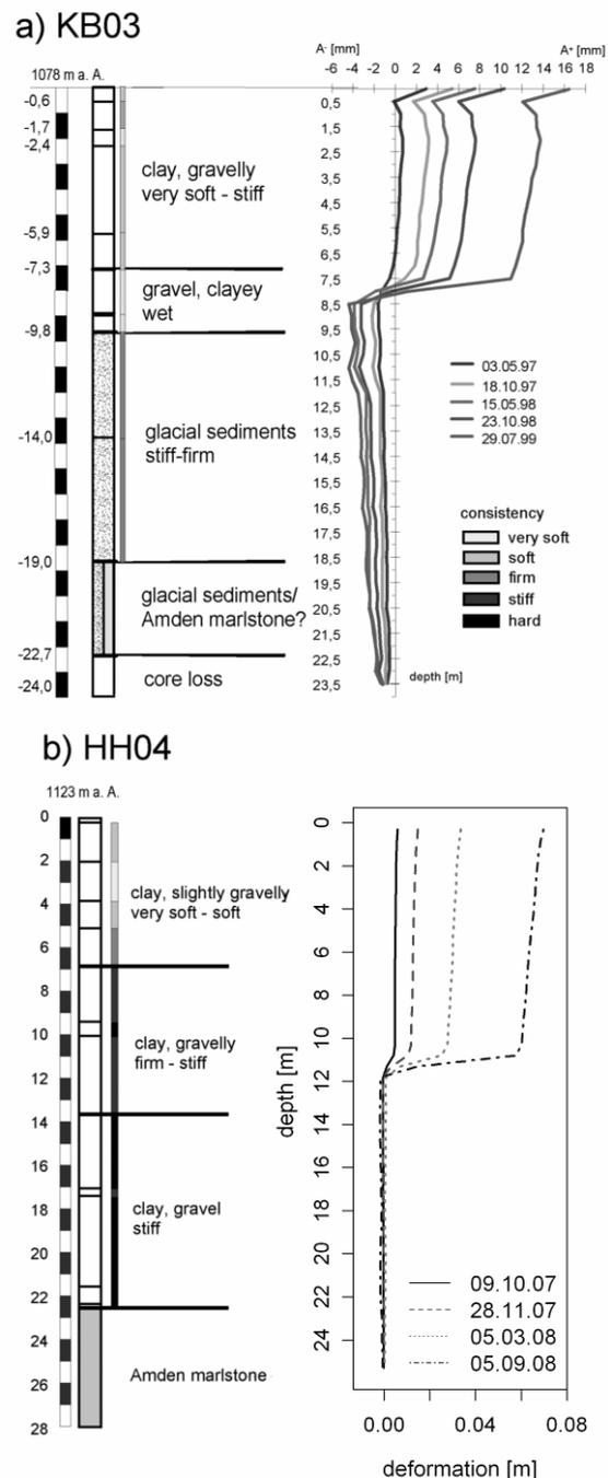
Figure 2. Borehole logs and slope deformation from inclinometer measurements at KB03 (a) and HH4 (b).
