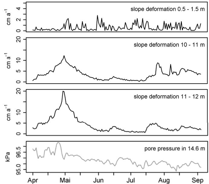
Figure 4. Maximum daily slope deformation rates at three depths at HH4 and median daily pore water pressure at 14.6 m at HH5 (hourly data from continuous monitoring in 2008).
