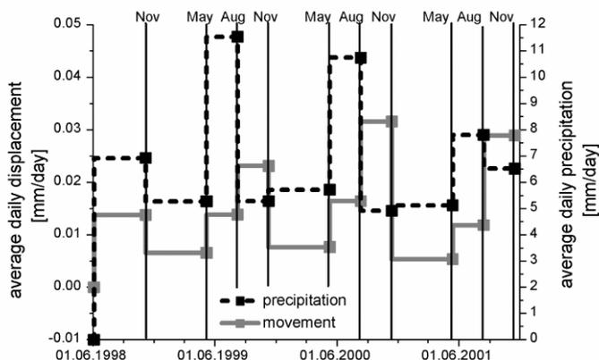
Figure 3. Average daily slope deformation rates from GPS measurements and average daily precipitation during the measurement intervals. Survey times are indicated by vertical lines.
