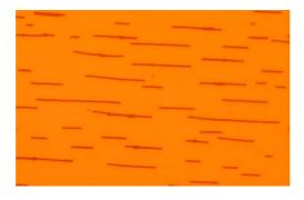
Figure 6. An example of the straight aggregates formed by 4  $\mu m$  spheres in 10 Oe magnetic field after about 2 hours.
