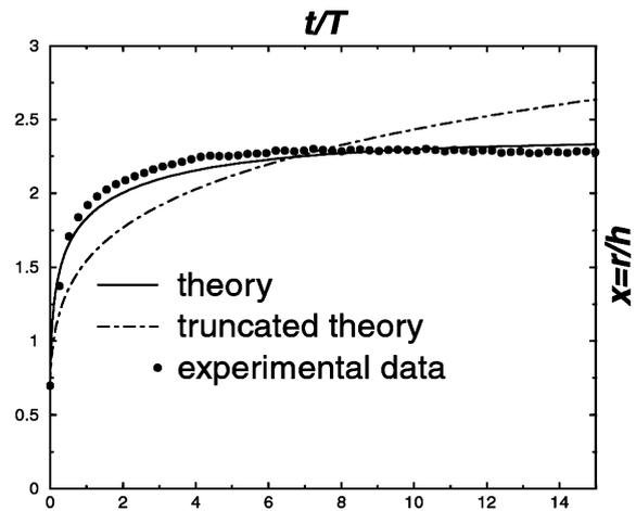
**Fig. 3** Scaled separation between a pair of particles as a function of the scaled time, comparison between theory and experiment obtained with an oscillating in-plane field of magnitude  $H_{\parallel} = 14.2$  Oe and a constant normal field  $H_{\perp} = 0.8H_{\parallel}$
