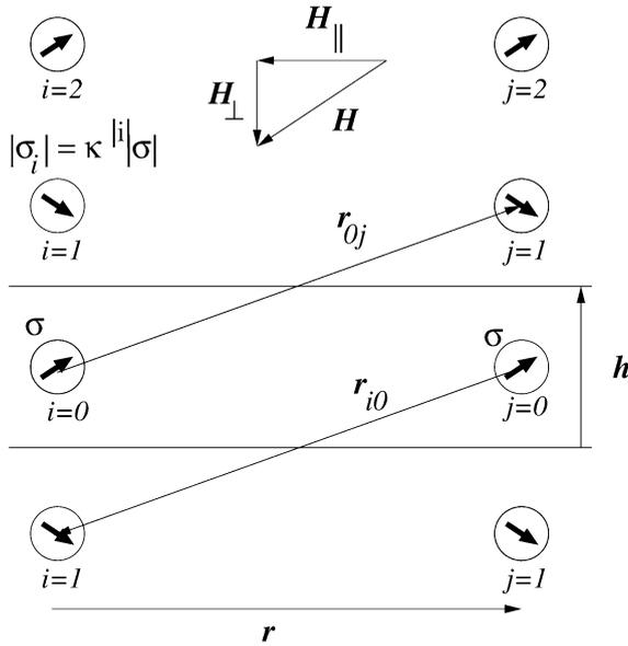
**Fig. 1** Pair of nonmagnetic particles in a ferrofluid layer, viewed along the confinement plates, and a series of dipole images accounting for the boundary conditions of the magnetic field along the plates
