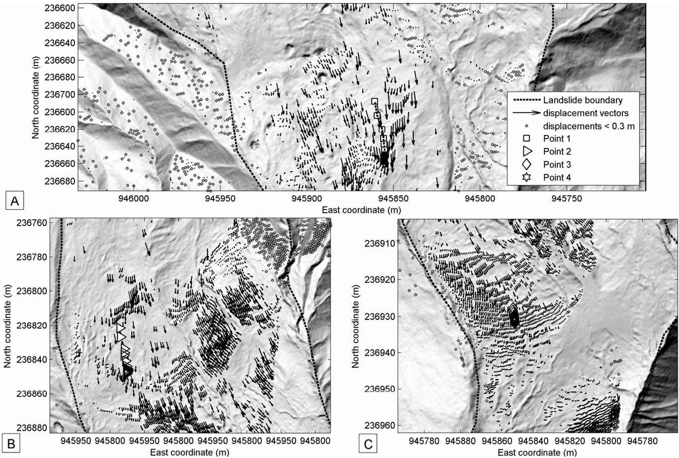
Figure 10. Displacement field for the 20<sup>th</sup> May 2008 in the local coordinate system in the upper part (A), in the middle part (B) and in the lower part (C) of the mudslide. The trajectories of the points 1, 2, 3 and 4 are also shown. Their cumulated displacements are presented in Figure 8.
