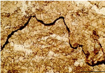
Micrograph of stylolite in Carbonate rock
