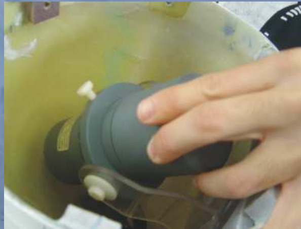
Aerodynamical bird (left) containing the cesium magnetometer (right)
