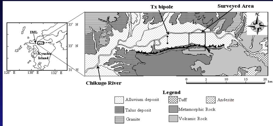
Geological map of the Minou fault zone (the rectangle restricts the CSAMT survey area; IML- Imari-Matsuyama Line)
