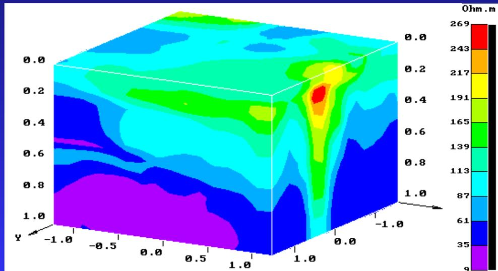
Resistivity model of the faulted area
